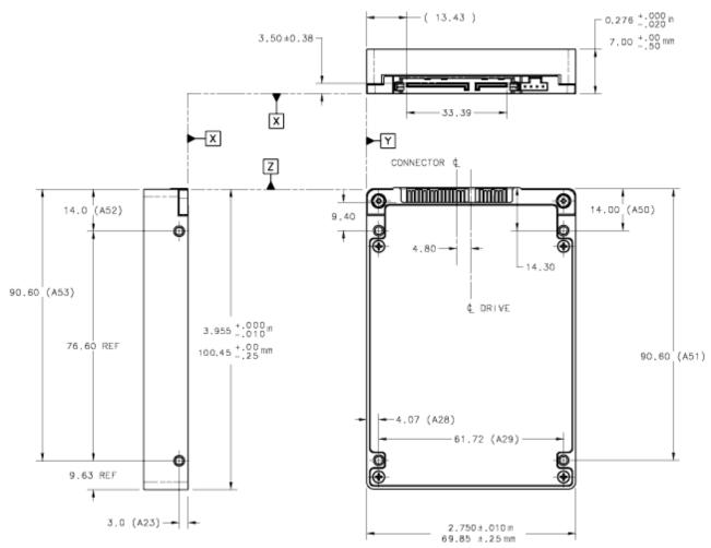
Figure 3. Mounting configuration dimensions (7mm models)
